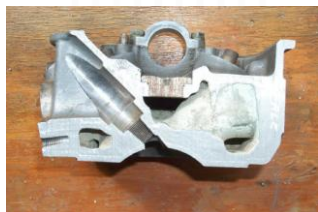
Ketelsteen in cilinderkop
